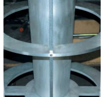
Waterjet cut rings, and cones prepared for powder coating
