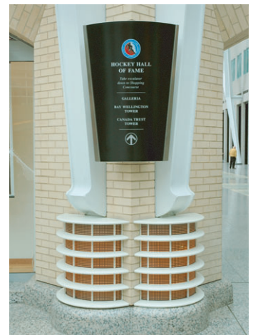
Shield sign made of brushed st. stl. and curved lexan graphic face
